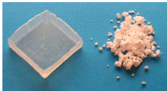
Figure 4. PS/PBA core-shell particles before (right) and after (left) processing at 25^\circ\text{C} under 5000 psi for 5 min.
